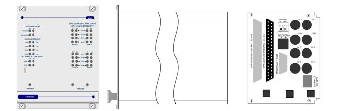
The **AMG4707AR** is a rackmount data transmit unit designed to transmit and receive up to 8 data or audio signals over two singlemode fibres. The 8 data/audio channel interfaces, whether RS232, RS422, RS485, 20mA, TTL, Contact Closure, Lonworks or Audio, are defined at manufacture by the addition of daughter boards fitted onto the Data Expansion Board A.
